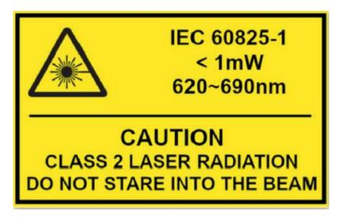
The Instrument produces a visible laser beam.
