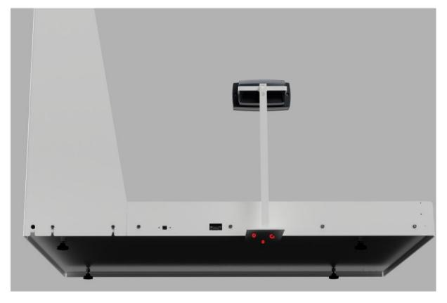
Install the 3 M5 screws to fasten the indicator to the base of the dimension scale.
